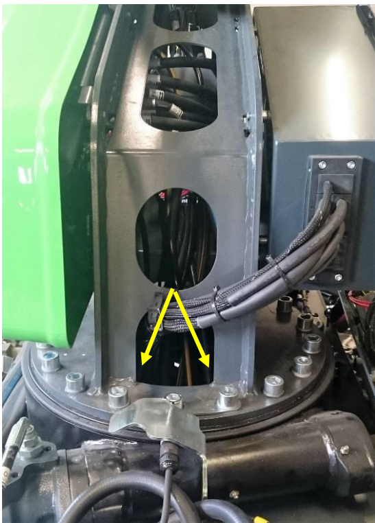
Greasing the slewing ring through the pedestal (2 grease nipples), pictured from the front.
