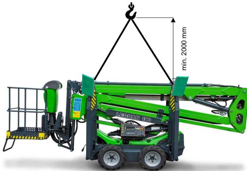
Figure 13 Lifting the access platform
