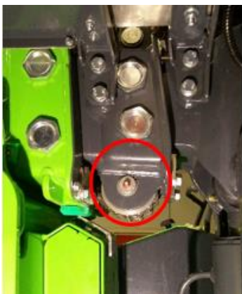
Figure 17 Telescoping chain pulley grease nipple
