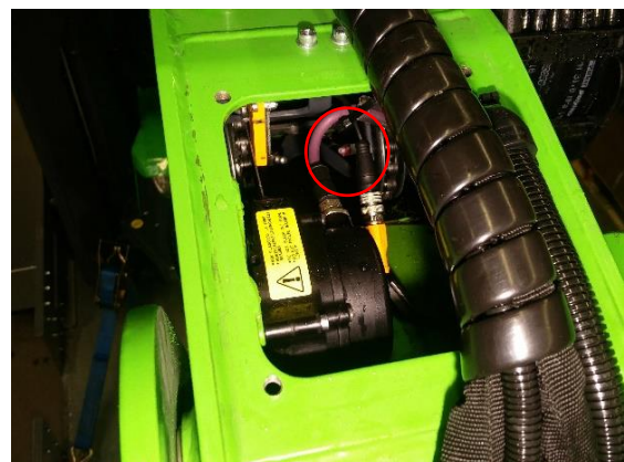
Figure 18 Leaf chain pulley greasing points in the front side of the 2 nd boom
