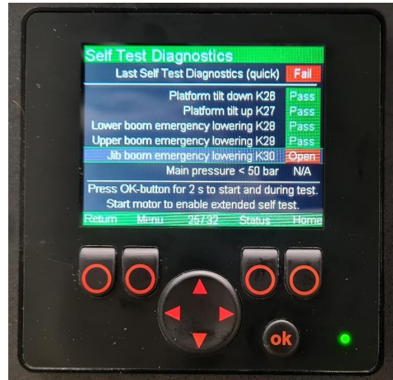
Figure 31. "Self Test Diagnostics" page error
