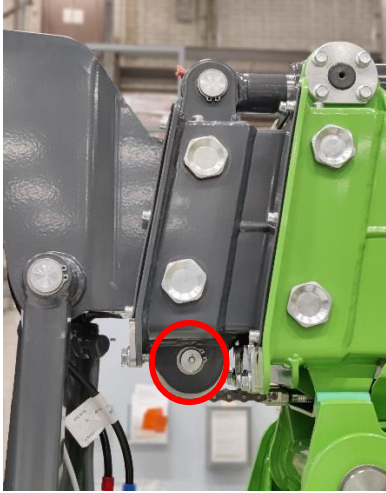
Figure 22. Telescope chain pulley wheel greasing point at the work platform end
