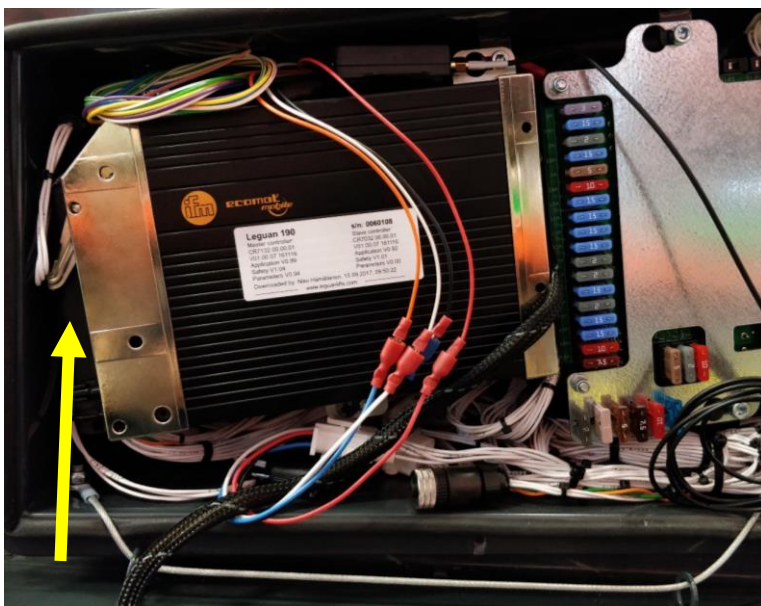
Figure 35 Contacts to the logic controllers (3 pcs)
