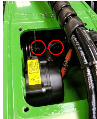
Figure 19 Leaf chain pulley greasing points in the front side of the 2nd boom
