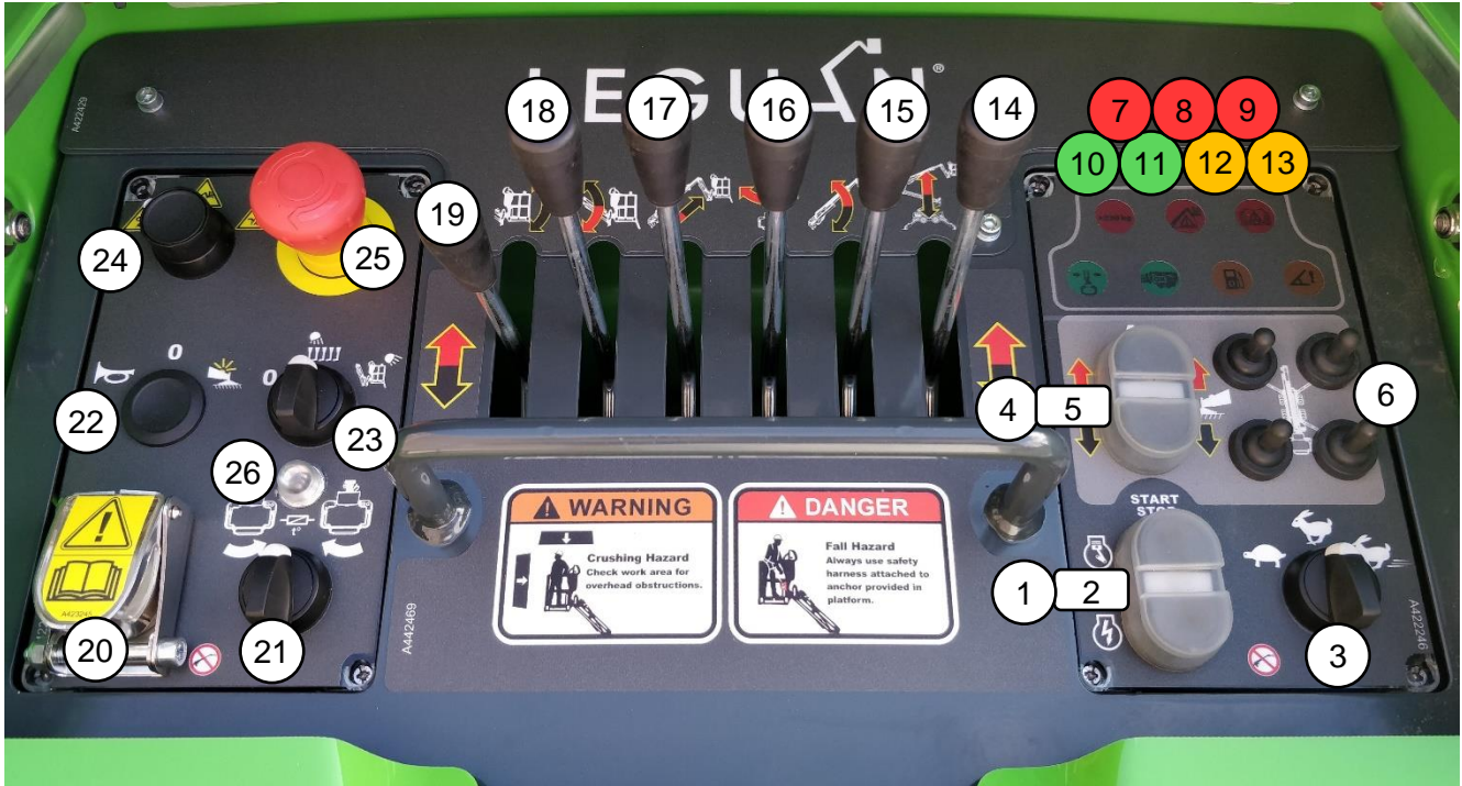
Figure 5: Upper control panel's levers, switches and buttons
