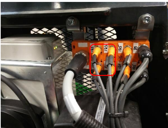
Figure 27 Splitter Box, outrigger connectors marked inside red square
