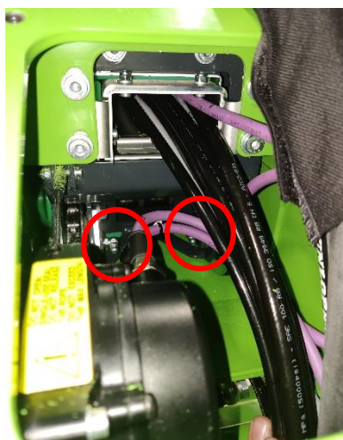
Figure 19. Telescope chain pulley wheel greasing points at the lower and upper boom linkage piece end
