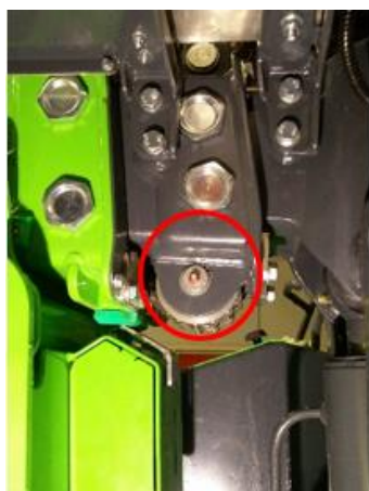
Obr. 11 Maznica remenice teleskopu
