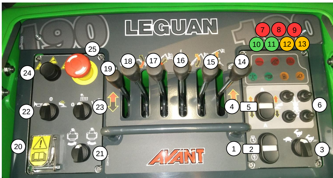
Figure 5: Upper control panel's levers, switches and buttons
